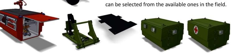
In case of the malfunction of the base vehicle the specialized superstructure module can be deployed within a short time using another carrier.
