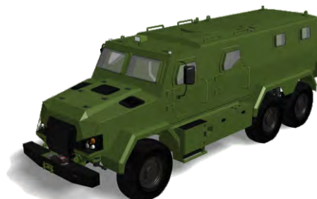
6x6 WD vehicle with monocoque armour body
