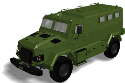
4x4 WD vehicle with monocoque armour body
