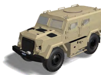
4x4 WD patrol vehicle with monocoque armour body
