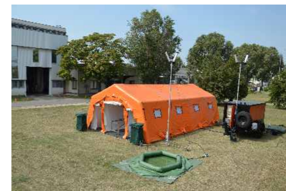
SZMF - personnel decontamination equipment
