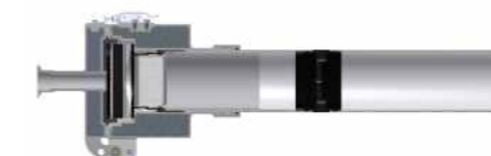
lead shielding for air monitoring (8)
