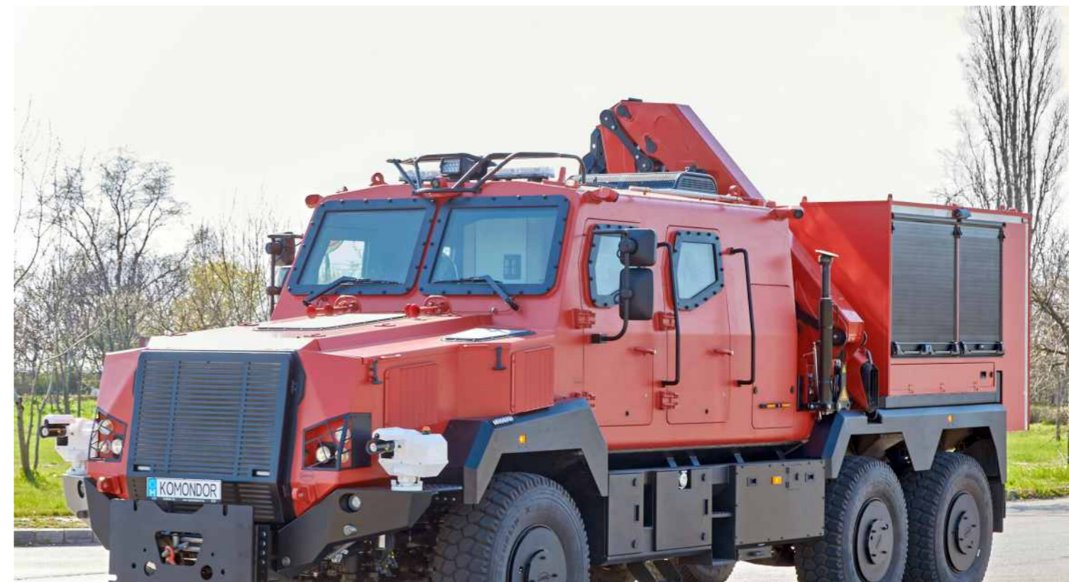
GMMF-20 Technical recovery superstructure: 11 t meter hydraulic crane Lift-tow fork with up to 8 t capacity
