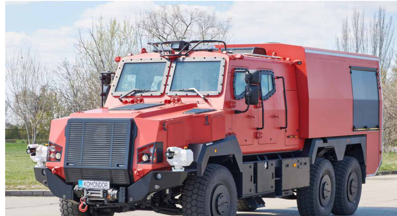
VCSF 7000 Firefighter superstructure: 7000 l water tank with fire-fighter pump Remote controlled front nozzles
