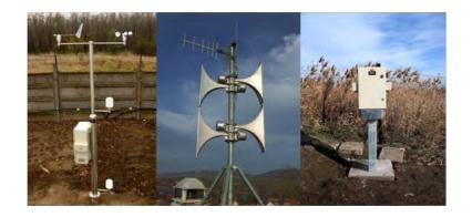
Reference 1: Telemetric and public alarm systems are implemented in the most dangerous 19 factories selected through risk analysis and 30 settlements around them in Hungary. The system consists of more than 300 monitoring stations and more than 500 public alarm sirens.
