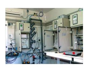
The on-line water quality monitoring system is capable of indicating the changes in water quality (parameters) and performing a variety of measurements in water on site. The monitoring system has an instrumentation with a wide measuring range to perform successful measurements and sampling either in clean water or in a heavily polluted canal.
