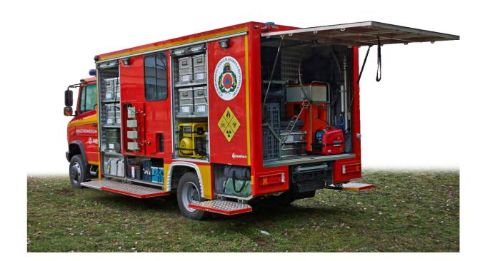
Using this equipment in full autonomy is not planned, so it requires external (230 V AC) power supply. Its collapsible water tank (1 000 or 3 000 L) can serve as a water source or it can be supplied from pipe system.
