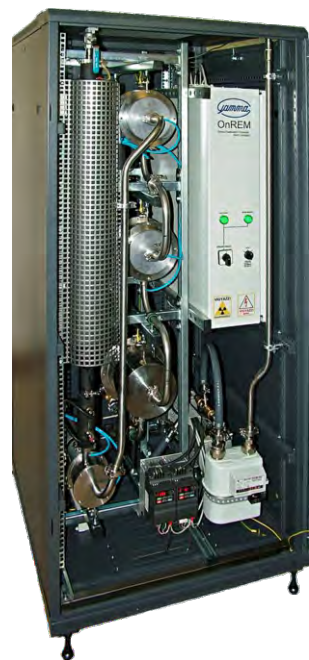
Measuring alpha, beta and gamma radiation emitting materials in gaseous or liquid substances
